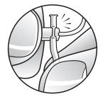
The wide part of the sports lock will snap out of place and the thin part of the sports lock will be positioned in the slit of the receiver end of the receiver tubing.
