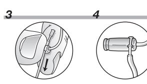
Place the receiver and sports lock between thumb and index finger and then pull the sports lock through.
