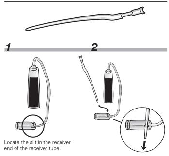
Slide the narrowest end of the sports lock into the slit starting from the side of the slit that is closest to the hearing instrument.
