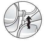
Hold the receiver in one hand and the sports lock in the other while pushing/wiggling the sports lock.
